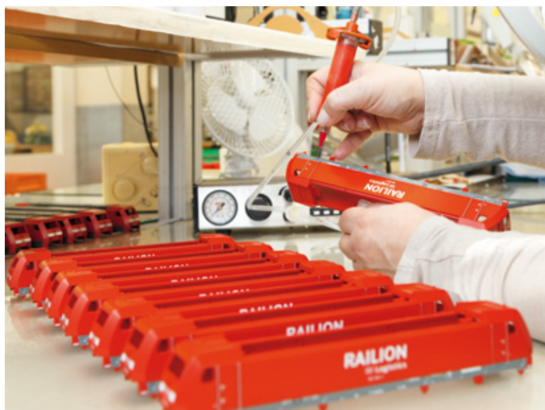
Uniformity: To color the recesses in the body-shell of the class 185.2 electric locomotive, a dosing machine with compressed air is used, and the amount of paint is always constant.
