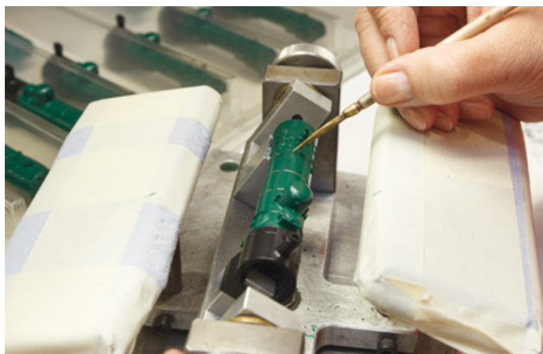
Accurate: To ensure the uniformity of the brush-stroke and color applied, the boiler of the SNCB class 98 steam locomotive is secured in the hand-painting shop in the hand-clamp.
