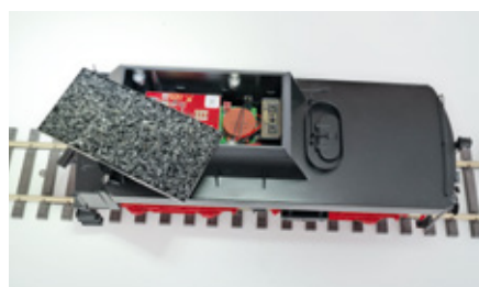
Tub-style tender: The multi-protocol digital decoder (Motorola, mfx, DCC) sits under the removable 100 x 49 mm (4 x 2") coal insert.
