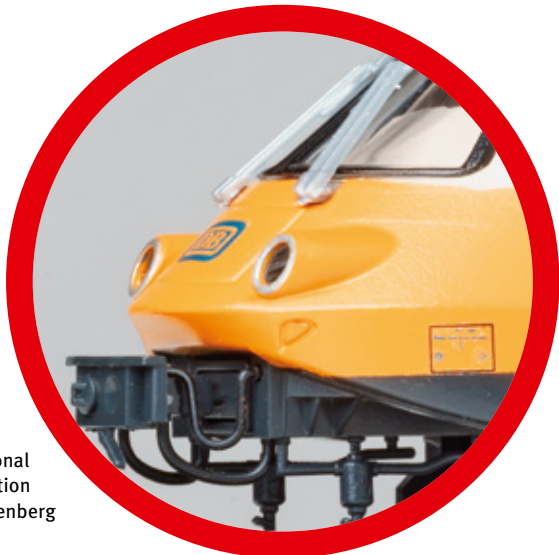
All there: Signal horn, antenna, catwalk and with braking resistor connected with side covers.
