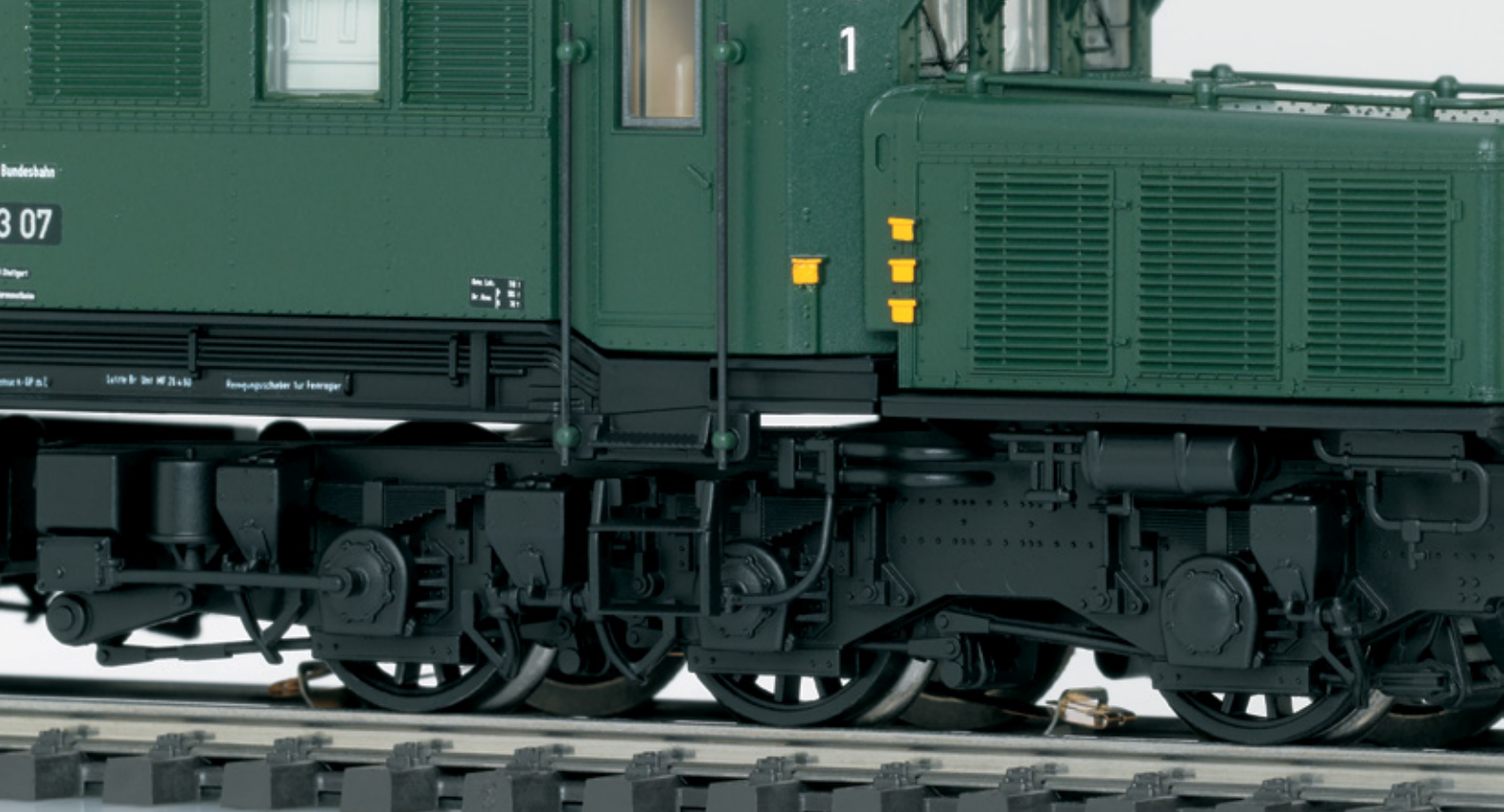
New design "German Crocodile": The authentic nature of the E93 07 in H0 is characterized by the painting, lettering, separately-applied parts and die-cast metal molding.
