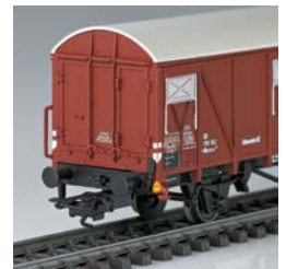
Detail car set 2 (see page 8): Representation of the three-section end doors of the Gltmmehs 62 boxcar.
