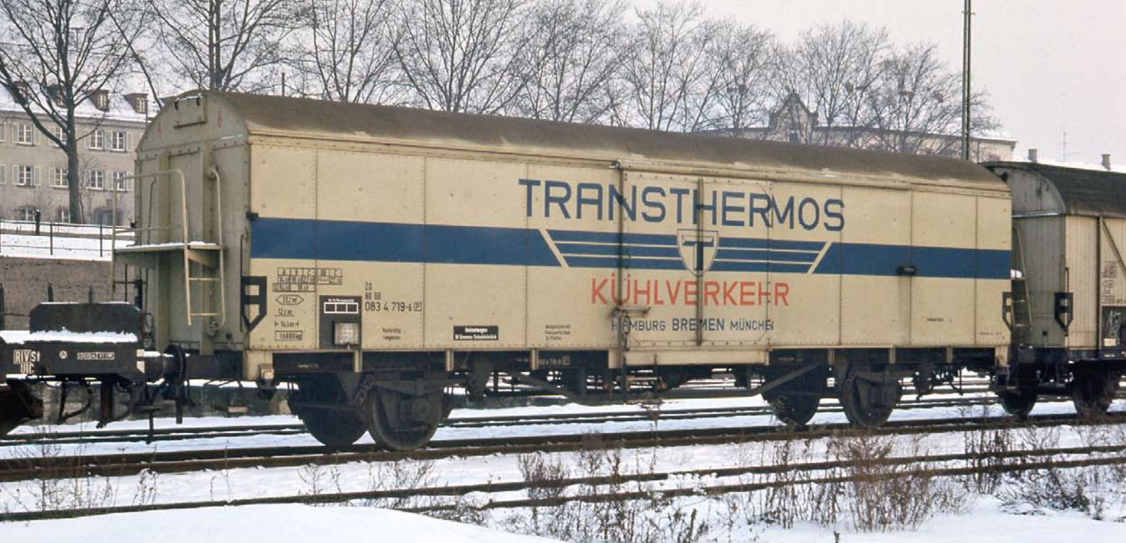
Insider H0 Annual Car: the mighty type Ibbblps 379 refrigerator car with work platform and dry ice chute was hired from the DB by Transthermos.
