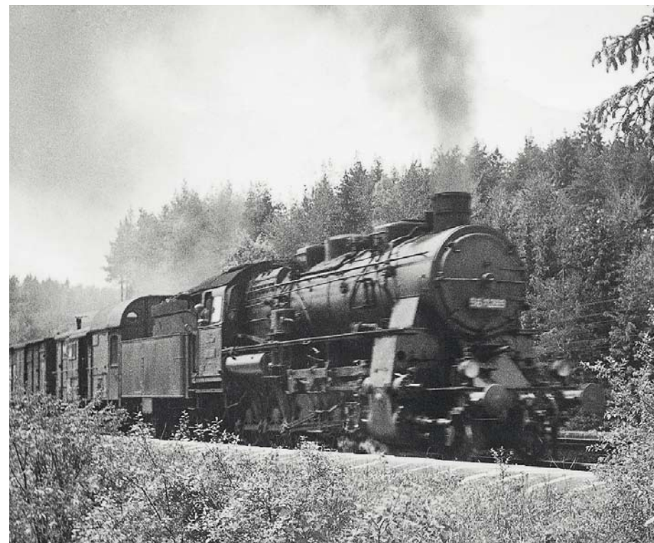
Striking class 58: the bulges at the top of the boiler ahead of the engineer's cab give away the presence of the squared-off Belpaire firebox; its shape allowed more space for steam production.
