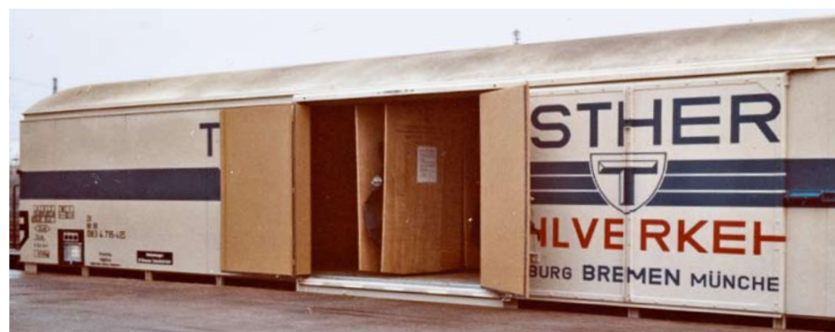
Insight: behind the open sliding doors of the Ibbblps 379 there are swing doors, so the heat-sensitive loads such as chocolate or margarine were always well insulated.
