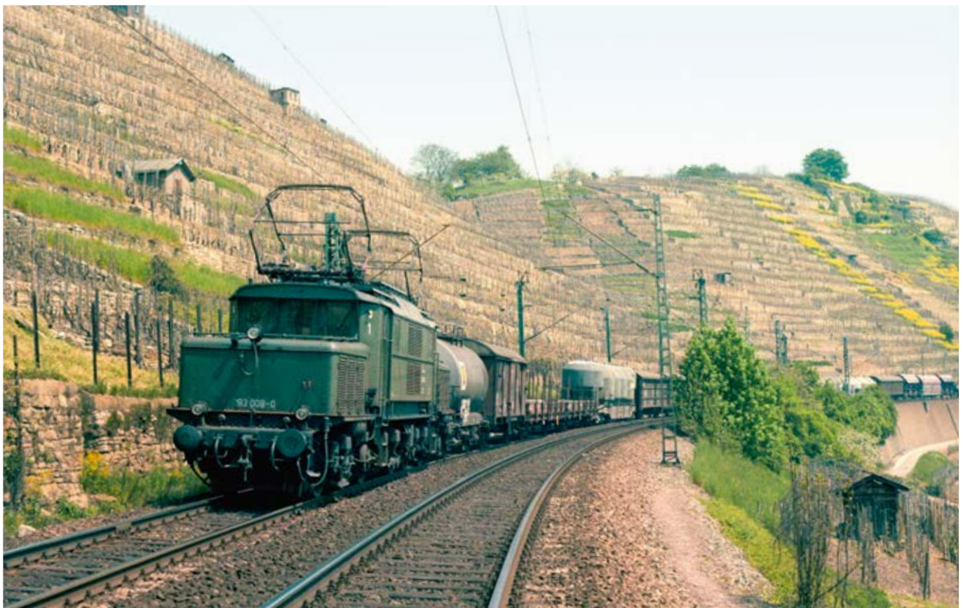
Enormous performances: Several of the E 93 locos covered over 13,000 kilometers (8,080 miles) a month hauling heavy freight trains.
