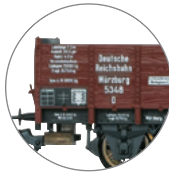
Type lesson "Om": The "O" stands for an open car (gondola), and the "m" stood in 1909 for a load capacity of at least 15 tonnes; this was raised in 1921 to 20 tonnes.
