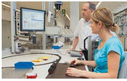
Boundary values: in the final inspection, the screen betrays whether functions of loco and tender are outside the narrow tolerance zone. The testing program, designed for the specific article,...
