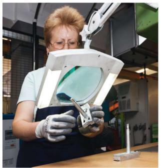
From a single mold: fresh from the casting system the swarf is still decorating the tender housing of the class 50.40, about to be minutely examined under the illuminated magnifying glass. Märklin's prizewinning zinc molding expertise ensures esthetic and tactile quality of the model.
