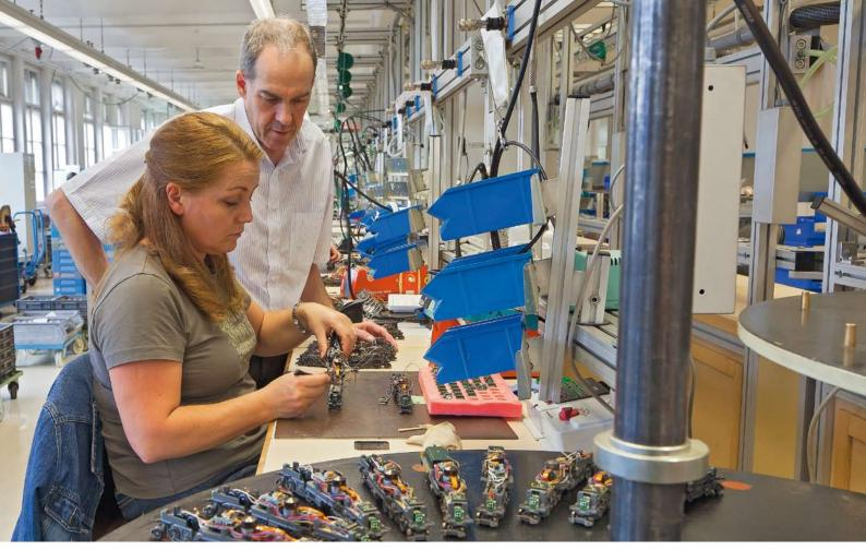
Last fitting station before the "wedding": the joining of locomotive chassis with its superstructure shows the finished model for the first time. Assembly is now complete - and is of course documented.
