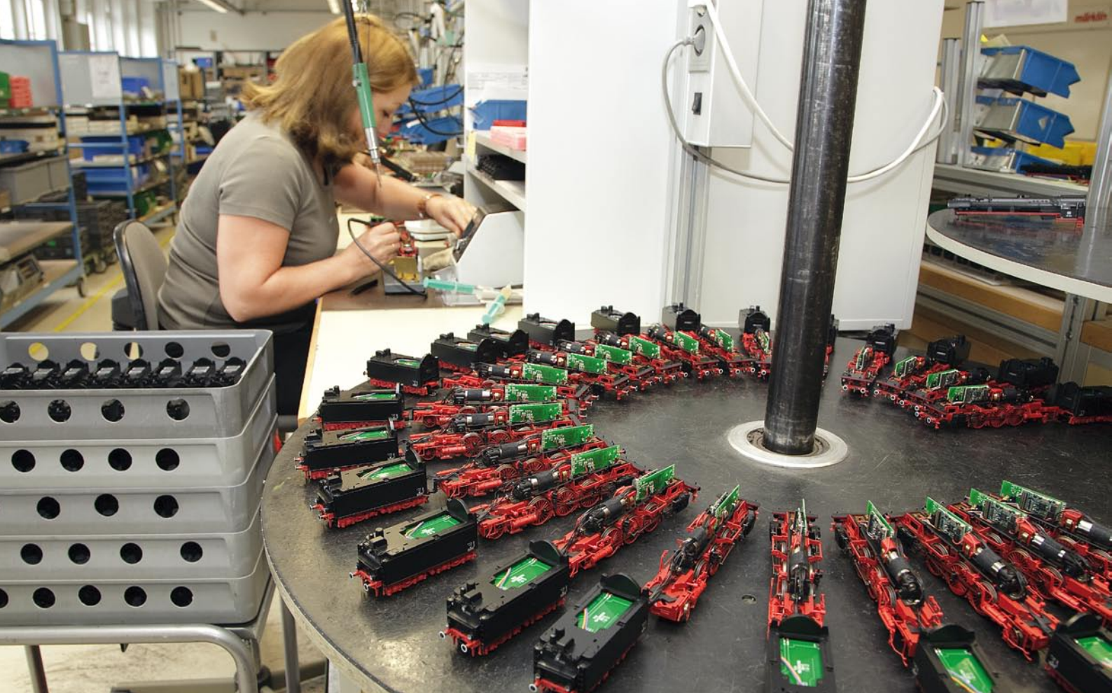
Gyro just before the ceremonious moment: The assembly department calls the connection between the lower and upper sections of the locomotive the "marriage". To be seen in the tender is the circuit board with the electronics for all the noise functions.
