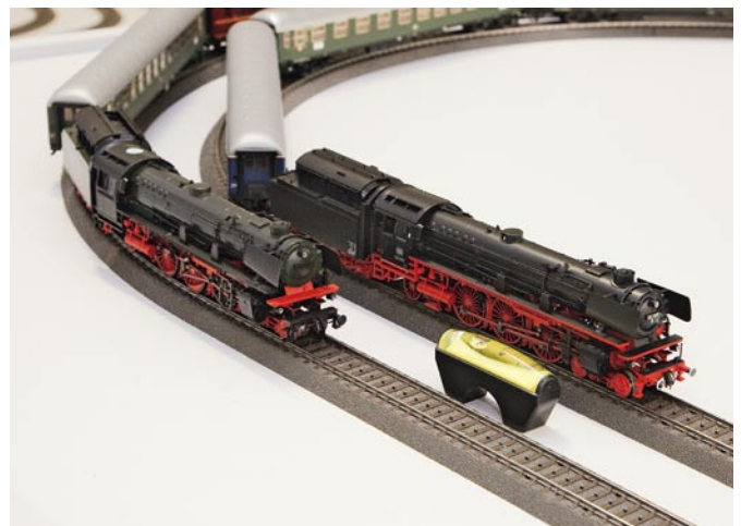
Hill-climbing test: in the test lab the analog-controlled class 03.10 (right) leaves the uncontrolled loco behind it on the climb.
