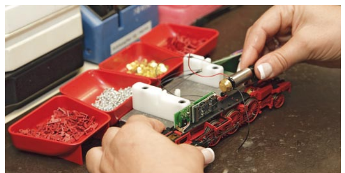
The bell-armature motor is then underneath the diecast boiler.
