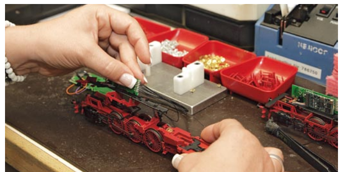
The circuit board with the electronics is carefully fitted to the lower section.
