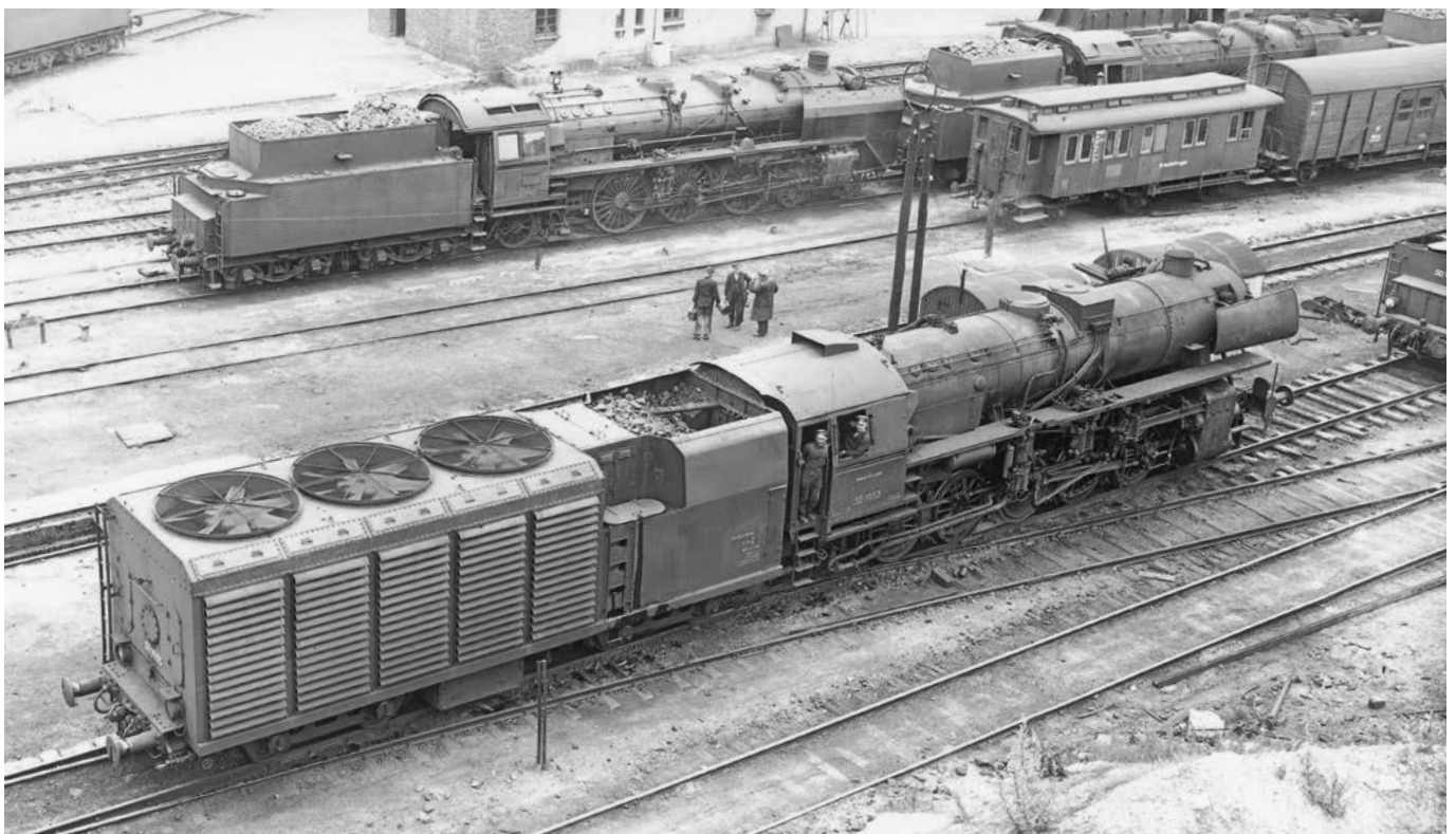
Overview: Here 52 1953 is caught shunting in Osnabrück depot in 1949. Clearly visible on the condensing tender are the ventilation fans and the shutters.
