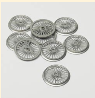
Step 1: In the pre-treatment section, the die-cast zinc component is cleaned. For this, an immersion process using ten-sides is used, or possibly also ultrasonic or electrolytic processes.
