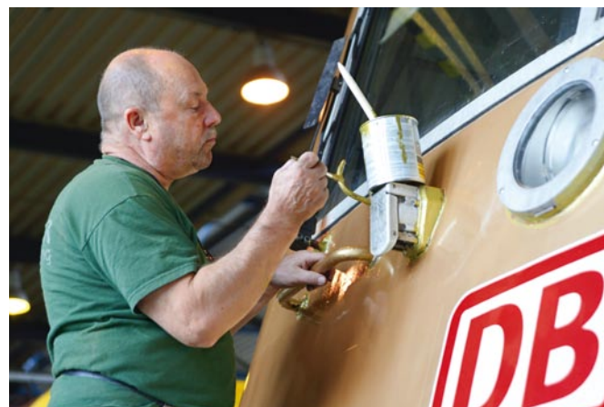
Precision work: Where the foil won't stick, the paintbrush comes to the rescue.
