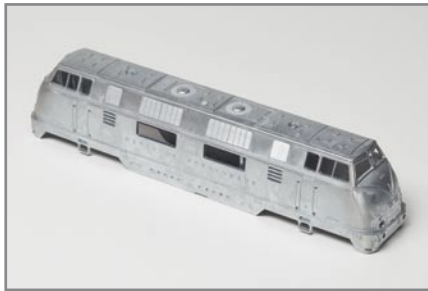
Before phosphating, the material surface of the zinc die-casting is cleaned in baths.
