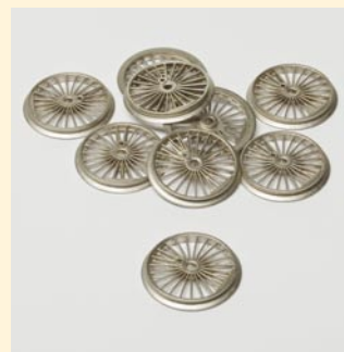
Step 3: In a further process bath, nickel is then applied to the component over the copper layer and this hardens the surface and also protects it from abrasion.
