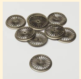
Step 4: Finally, black nickel is applied to the components as a decorative layer, and the depth of color can be precisely regulated.
