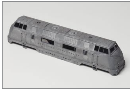
In the phosphoric acid bath a two-micrometer thick layer of zinc phosphate is formed.
