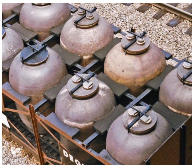
Withstand even the strongest of acids: the pots are made of stoneware.
