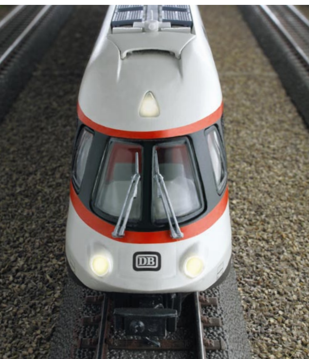
Aerodynamic: the very flat sloping front of the end cars of the class 403 favors its running behavior on high-speed lines to a remarkable extent.
