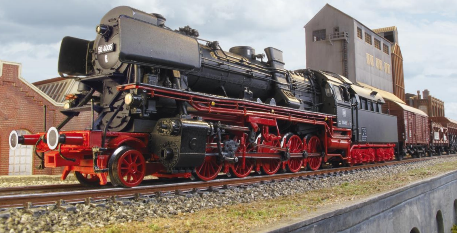
Phenomenal: two boilers, smoke-stack to the side, tender with moveable coal bunker covers – as the 2011 Club model, the Franco-Crosti class 50.40 loco impresses you with its unmistakable profile. Apart from that, the imposing era III steam locomotive stands for technical refinement.
