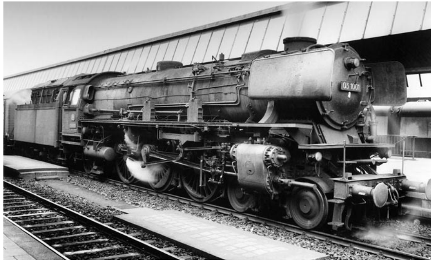
Dynamic Look Ensured: The Witte smoke deflector plates of the BR 03.10.
