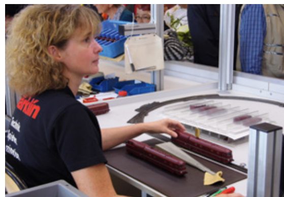
Final inspection: Before 05 003 is packaged, every model is subjected to functional testing.
