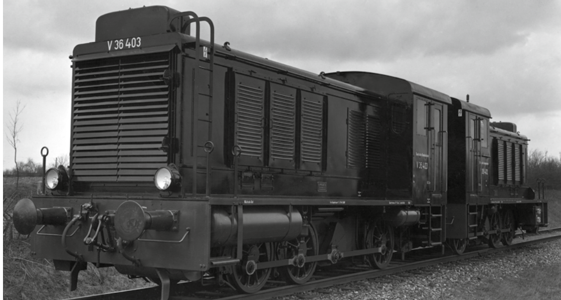
Double loco control: two locos of class V 36.4 coupled cab-to-cab.
