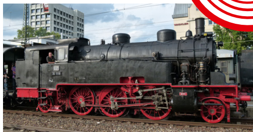
Guest at the IMA/Märklin Open Days 2017: The UEF loco 75 1118, a Baden VIc loco with welded water tanks.
