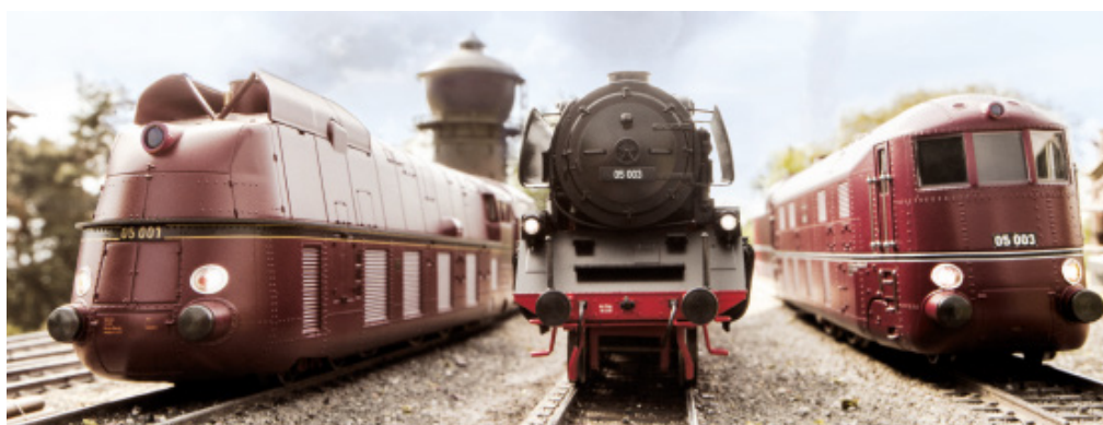
Worth a try: One of the three class 05 locomotives set a world speed record on a test run. Experiments were carried out with streamlined fairings and a front engineer's cab (far right).
