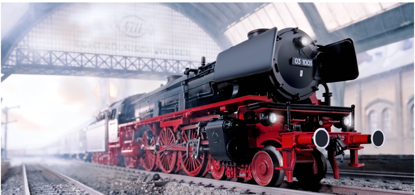
Reaction to accelerated express traffic: The two-cylinder standard locomotives of class 03 lack smoothness of running in higher speed ranges, so the designers conceived the three-cylinder locomotive of class 03.10. The DB designed 03 1001 with a new boiler.
